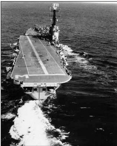
HMAS Melbourne (11) 5.5% angled flight deck.
