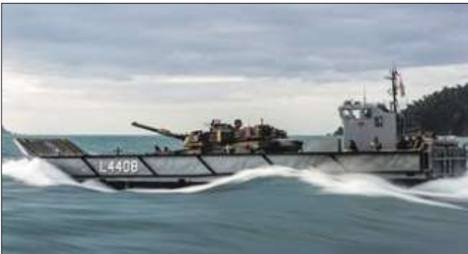
A light landing craft transports an M1A1 Abrahams to land as part of load trials.
