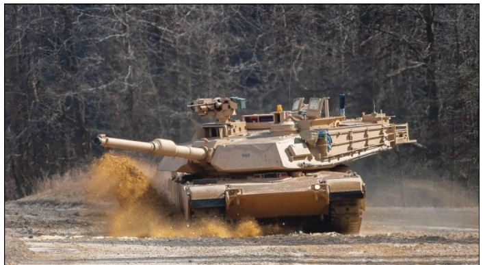
The M1A2 Abrams System Enhancement Package V3 is one of two upgrade options Army is considering to replace the M1A1 main battle tank
